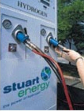
A hydrogen pump.
